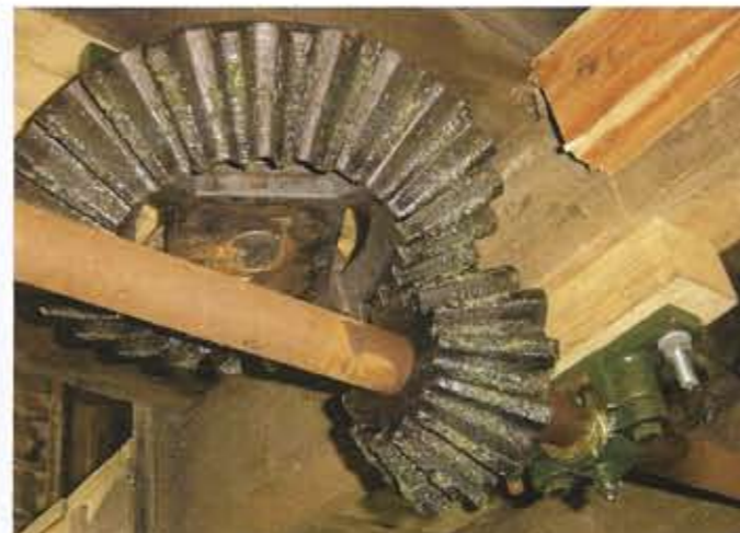
Phase 2 of the restoration project involved the casting of numerous cogs and fittings
